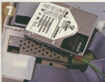
7 The IDE connector can now be plugged in and an insulating plastic pad is placed over the metal shield
